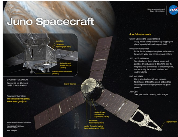
Juno spacecraft and its science instruments. Image credit: NASA/JPL
